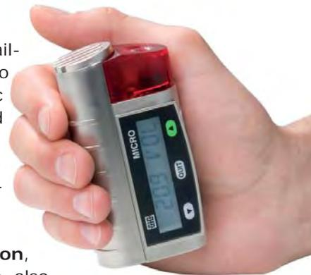
A **data-interface station**, and **docking station** are also available which make bump testing, calibration and data management significantly easier and save the user time and money. The Micro IV has an IR interface for fast and simple data transfer.
